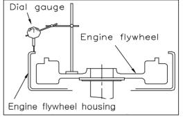
[FIG. 5-6] FLYWHELL HOUSING FLATNESS CHECKING
