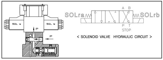
[FIG. 4-2] OIL FLOW OF STOP
