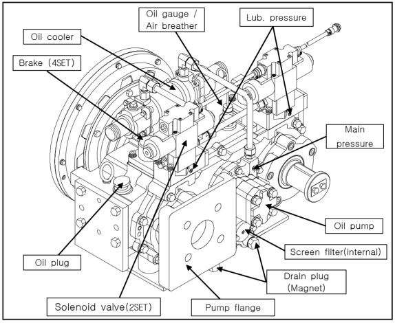
[FIG. 2-2] PTO external structure
