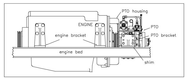
[FIG. 5-10] PTO INSTALLATION TO AUXILIARY ENGINE
