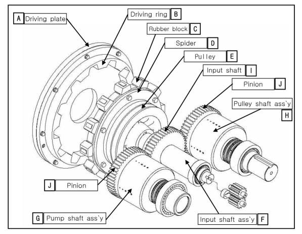
[FIG. 2-1] PTO Internal structure
