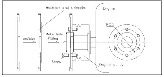
[FIG. 5-1] Fitting Dummy plate
