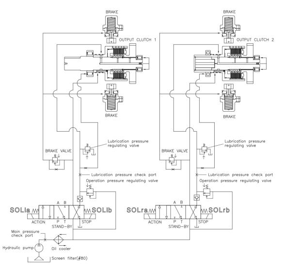
[FIG. 4-1]HYDRAULIC CIRCUIT DIAGRAM
