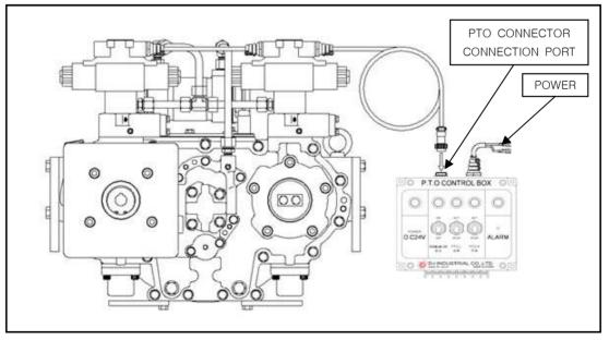
[FIG 3-2] PTO WITH ELECTRIC VALVE / CONTROL BOX
