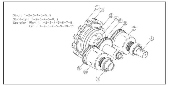
[FIG. 3-1] Power Transmission flow
