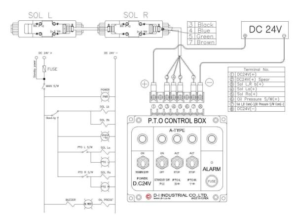
[FIG. 5-13] The wiring connection of control box and eletrical circuit diagram
