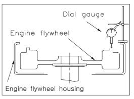
[FIG. 5-8] FLYWHEEL FLATNESS CHECKING
