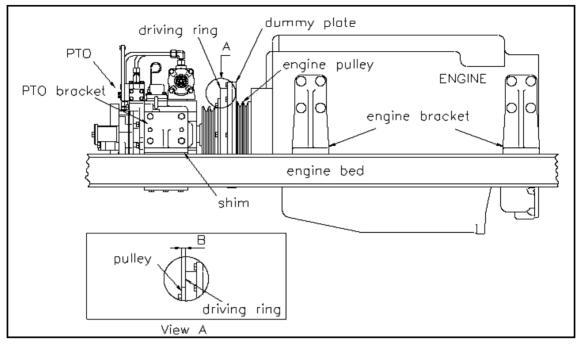
[FIG. 5-4] PTO installation
